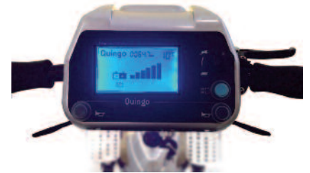
Multi-feature digital dash/LCD display with easy read user controls
