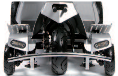
Quintell™ Self Centering Steering Defaults to straight travel with minimal effort
