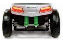
SmoothDrive II Suspension + LED lights Smoother,safer journeys with high intensity front and rear, hazards and brake lights
