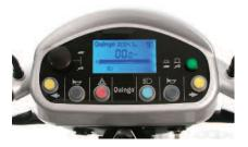
Multi-feature digital dash/LCD display Easy to read layout and controls
